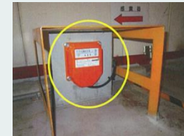
Rope misalignment stop
